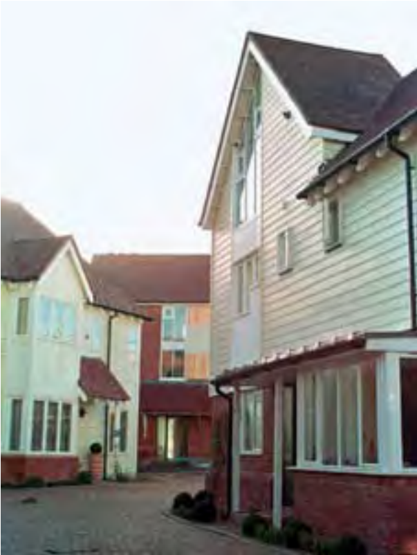
The skilful layout of buildings can ensure that windows of habitable rooms create oblique views rather than face each other.
