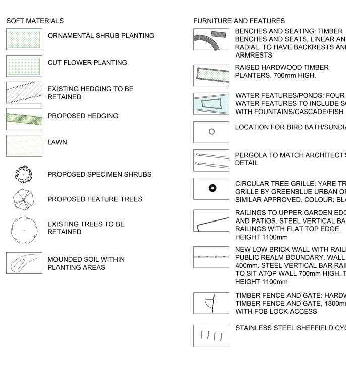
BENCHES AND SEATING: TIMBER BENCHES AND SEATS, LINEAR AND RADIAL. TO HAVE BACKRESTS AND
