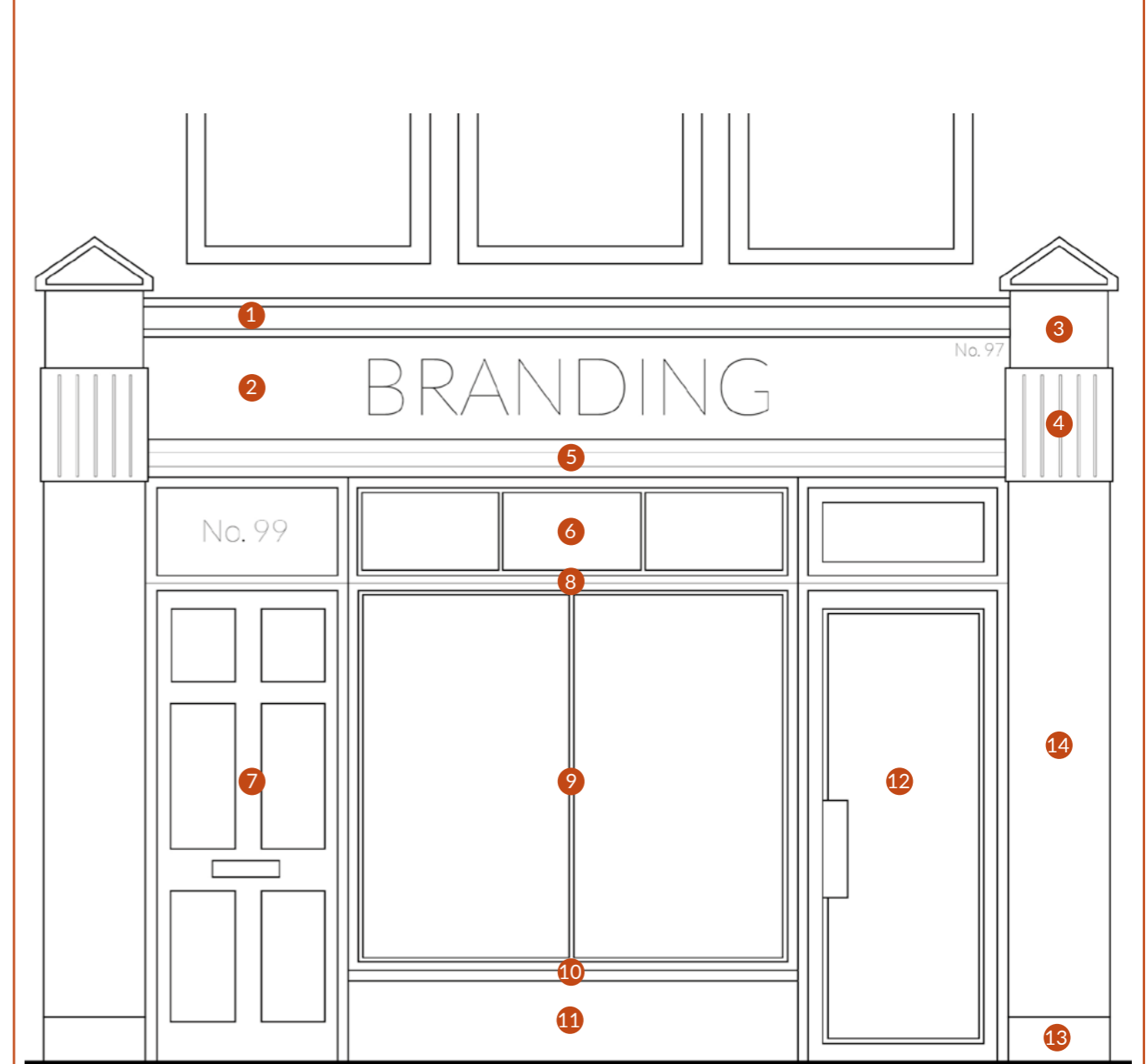
Fig.25 Key architectural features of a shop front
