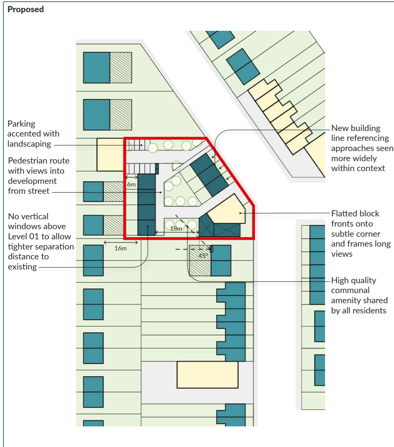
Fig.30 Proposed site plan showing new development made up of a range of typologies suited to their site specific constraints, with segregated access (car/pedestrian) and shared amenity landscape.
