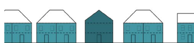
Fig. 10 In an area categorised as Maintain , where there is a consistent character, new developments should generally follow the parapet/eaves and ridge heights of the surrounding developments.
